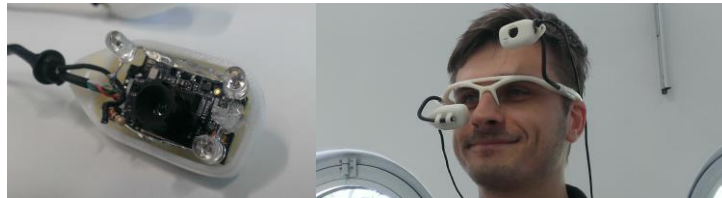
Figure 1: Prototype of a 3D printed open source gaze tracker
